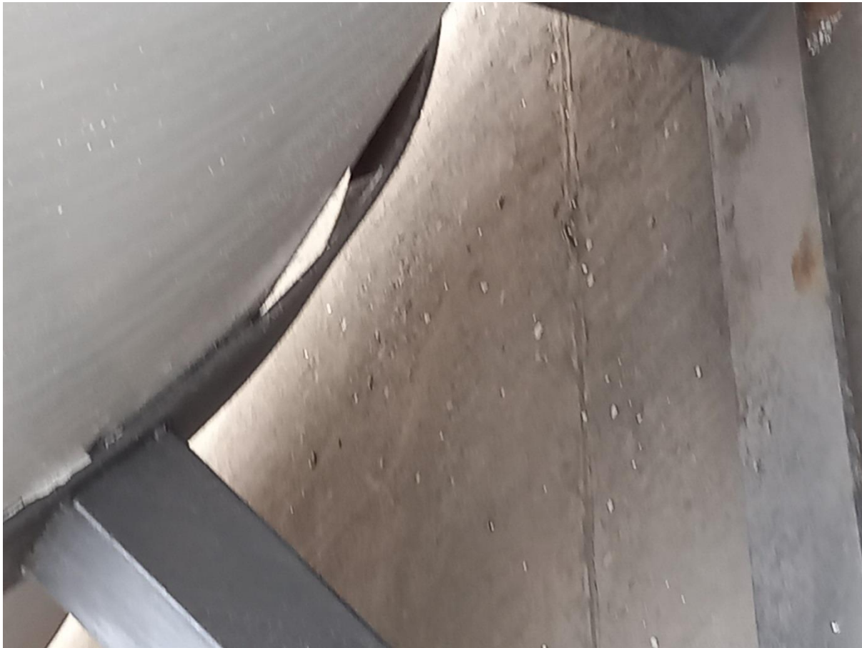
Vessel is not welded to the support
